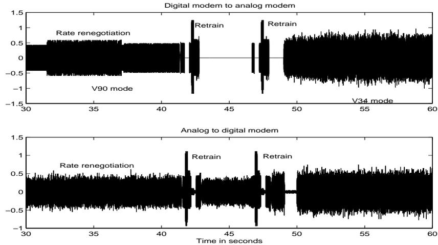
Figure 6: A real example of repeated rate renegotiation and retrains. Further explanations of the figure are in the messages from SMPA shown in the text.
