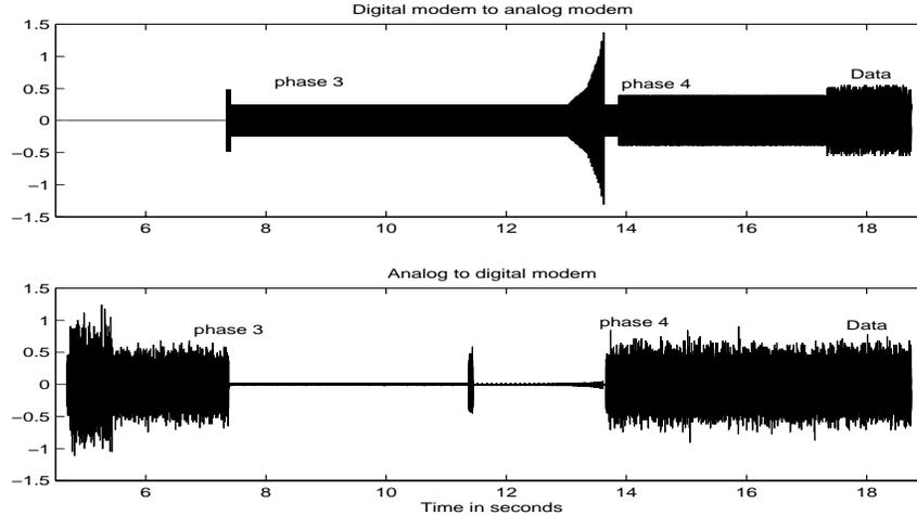
Figure 3: An example of phase 3 and phase 4 signal sequences. In this example, the downstream (from digital to analog at the top) has been selected during phase 2 to be V90 mode. If V34 mode were chosen, the signal sequence would look different, but similar to that shown in the bottom for the upstream direction where V34 mode is always used.
