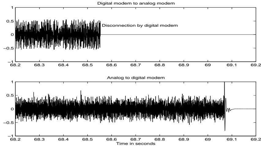
Figure 5: An actual example of the modem disconnection sequence.
