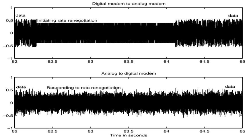
Figure 4: Rate renegotiation signal sequence. In this example, the downstream uses V90 mode. If V34 modem were chosen, the signal flow on top would look different (similar to that at the bottom).
