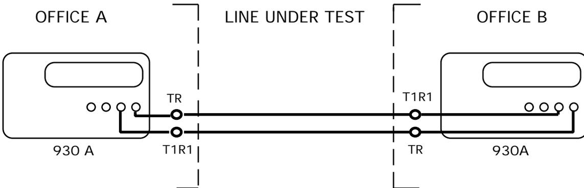
For 2-wire measurements only, the Tip/Ring connection is used. For 4-wire measurements the Tip1/Ring1, as well as the Tip/Ring, connection is used. The above test set-up works for Loop Start, Ground Start, Reverse Battery and SF supervision trunks.
