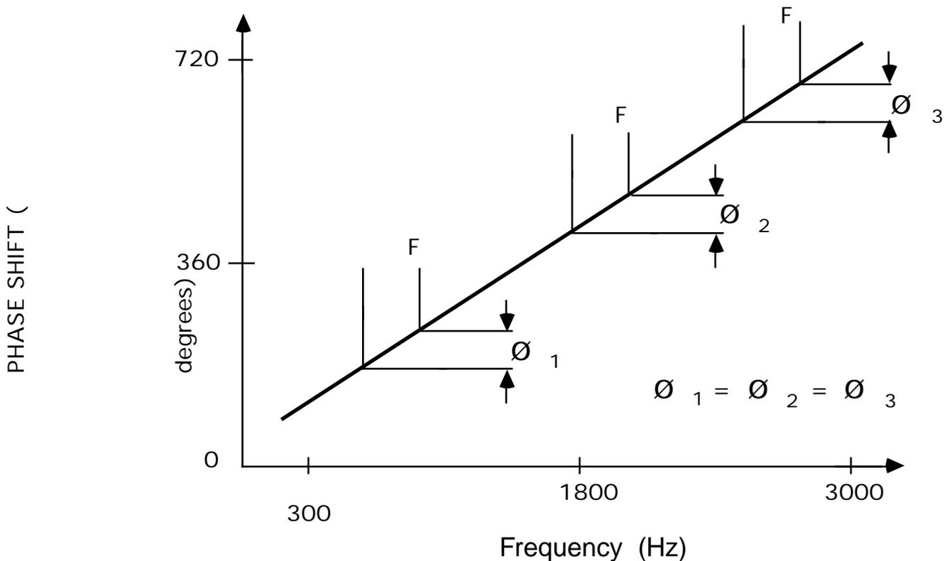
The phase difference  $\phi$  for a constant change in frequency  $F$  is the same anywhere along the above characteristic. In such a case, the envelope of the modulation would be delayed by a constant amount over the same frequency range as the carrier frequency was changed. The
