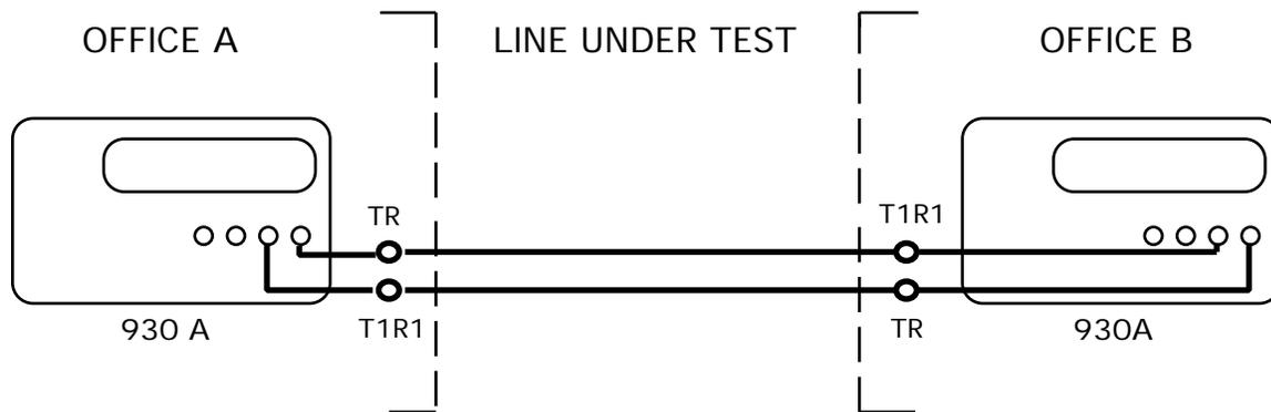
To set-up the 930A for signal-to-noise measurements, perform the following steps:
