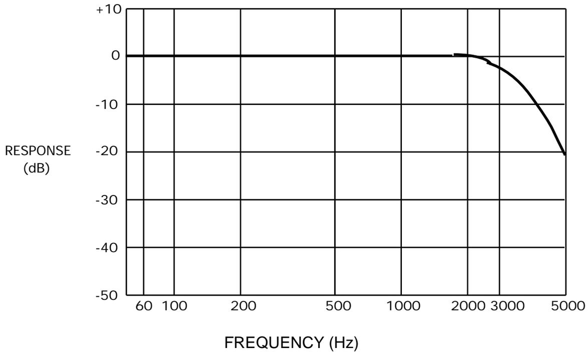
Compared to the C-Message filter, the 3 kHz Flat filter allows the low frequency noise contribution to be measured. By switching between C-Message and 3 kHz Flat filters, various sources of noise may be identified by their characteristic frequency bands.
