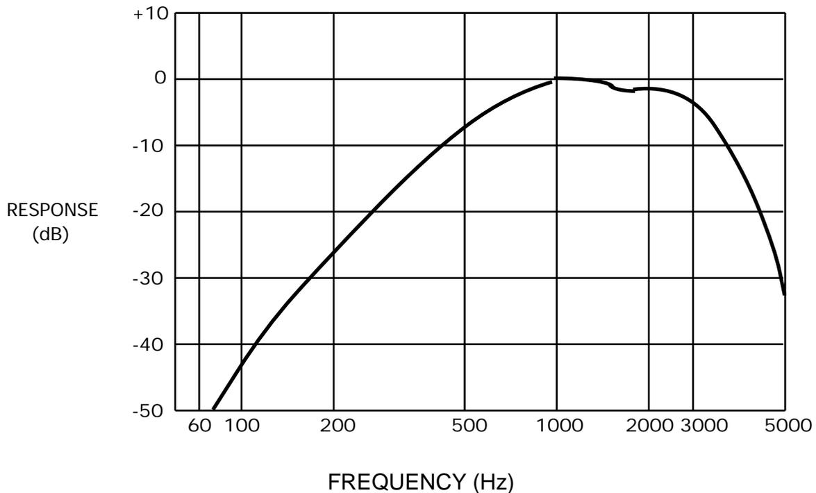
The C-Message filter is used to measure noise which affects voice communications and is not particularly relevant to data transmission. The 3 kHz Flat Weighted filter characteristic shown below more closely approximates the response of modems.
