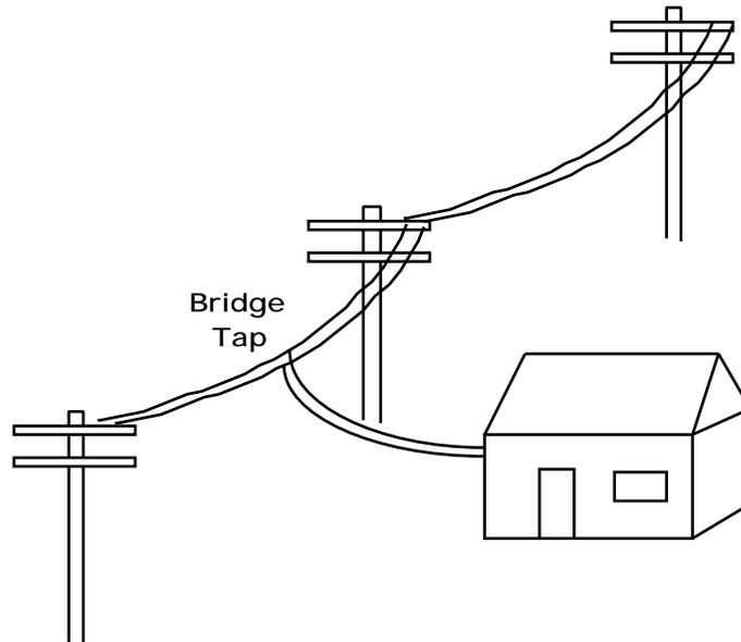
When service is disconnected, the wires are left in place but are unterminated. The capacitance these unterminated wires present to the circuit can produce significant phase distortion. Conditioned lines have all bridge taps removed. However, a regular dial-up call cannot be sure that bridge taps are not present. This limits home computer users to less than 1200 bps modems more than any other factor, with the possible exception of load coils which are discussed next.
