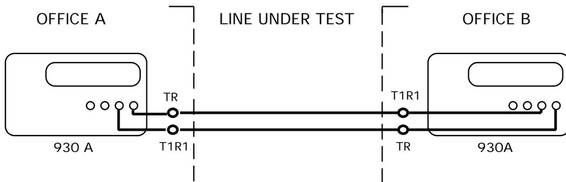
1. Repeat the 1004 Hz Loss measurement performed in the previous section. Send 1004 Hz at -16 dBm0 from Office A.
