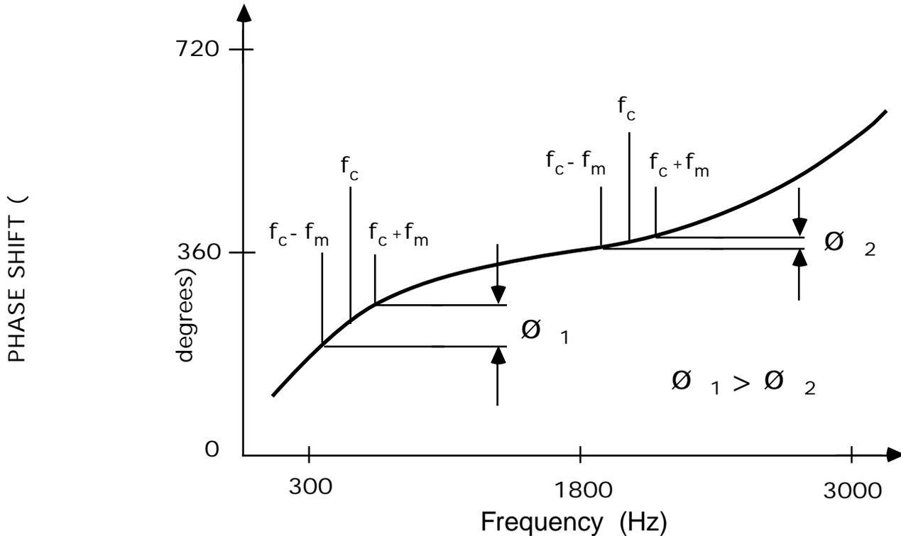
From this diagram it is apparent that even though the modulating frequency has remained the same, the phase difference has not remained constant as the carrier frequency changed.
