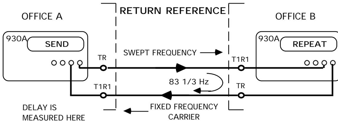
Select the correct trunk type as described in Section 3-4 of the 930A Manual and connect the 930A as described in Section 3-4.4. Complete this step before proceeding.
