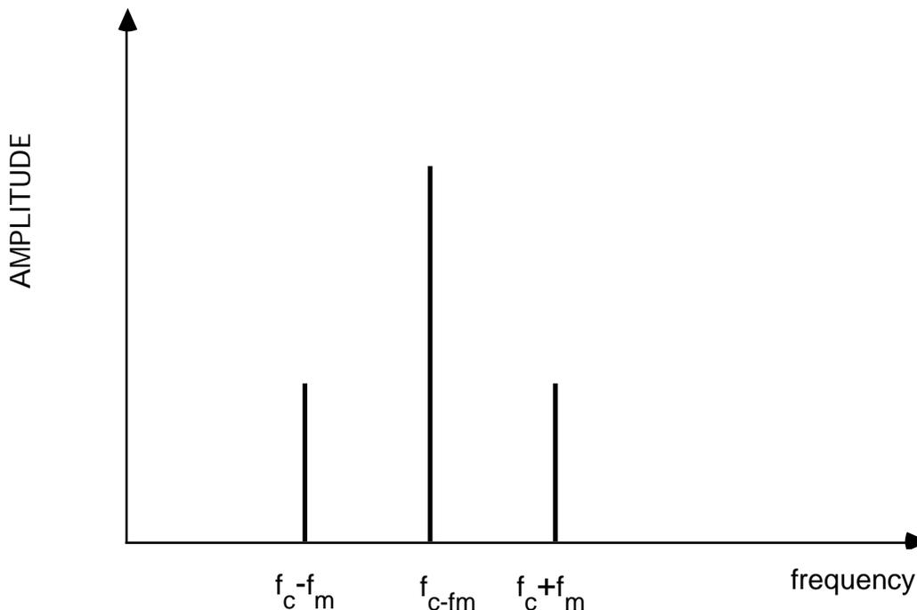
Amplitude Modulation produces a spectrum, such as that shown on the previous page, composed of the carrier frequency ( $f_c$ ) plus an upper and lower sideband ( $f_c+f_m$ ,  $f_c-f_m$ ). The modulation contains the information being transmitted by the AM signal. In this case, the information is the phase shift or delay difference between the modulation envelopes of the upper and lower sidebands.
