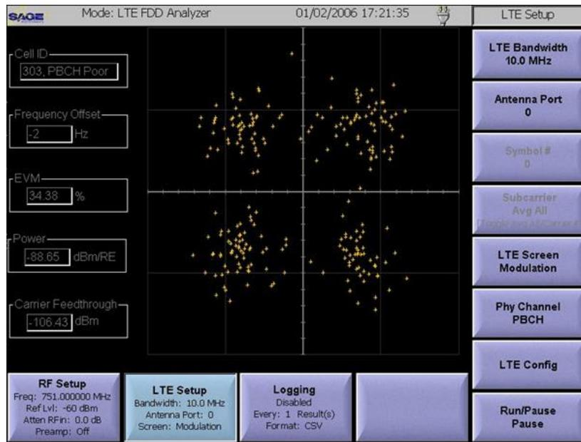
*Figure 2 Shows the PBCH Poor condition (meaning there are bits errors, but still correctible, marginal performance). This signal was obtained using an Omni antenna at an indoor location about ½ mile from cell site..*
