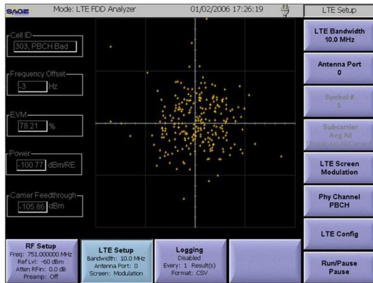
*Figure 3 Shows PBCH bad Condition (meaning there are uncorrectable bit errors). This signal was obtained using an Omni antenna about 3 miles away from the serving macro-cell.*
