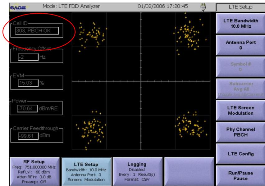
Figure 1 Shows the PBCH constellation when the PBCH is OK (meaning no bit errors). This signal was obtained using an Omni antenna about one mile from the cell site and roughly in the center of a sector.
