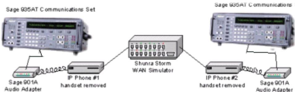
**Figure 1 -- Test Setup, IP Phones Speech Quality Test**
