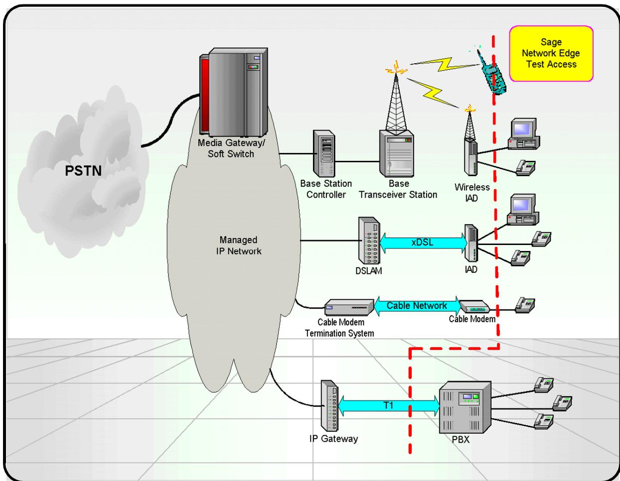
**Figure 1** — Sage Test Access Points at Network Edge
