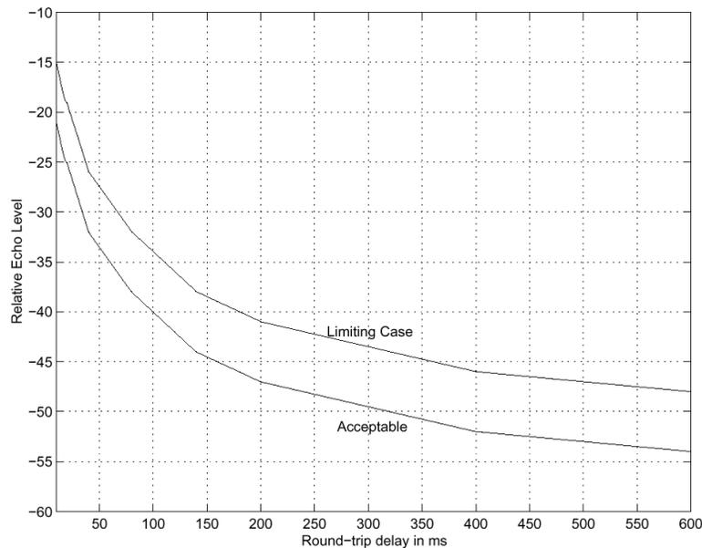
**Figure 2** — Echo Tolerance Curve
