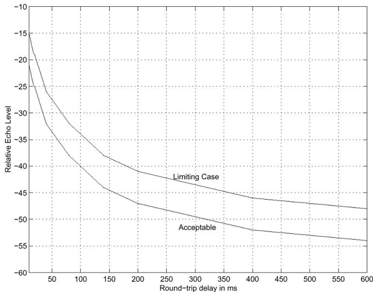
**Figure 2** — Echo Tolerance Curve
