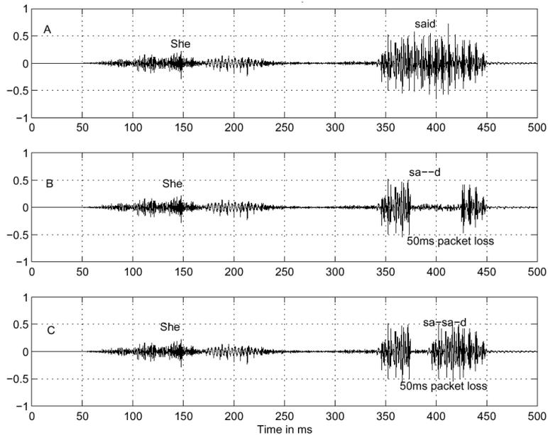
**Figure 3** — Packet Loss Examples
