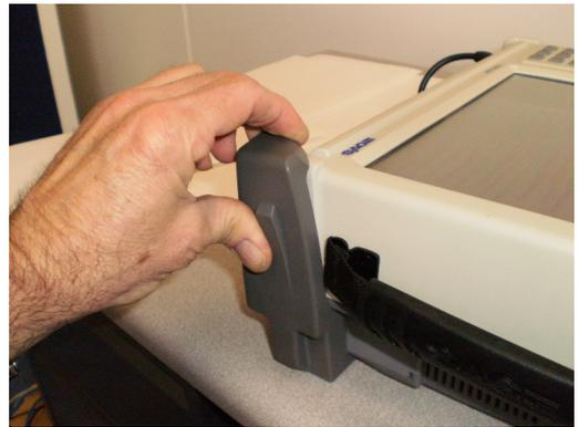
Figure 2.8 Removing Corner Protector
