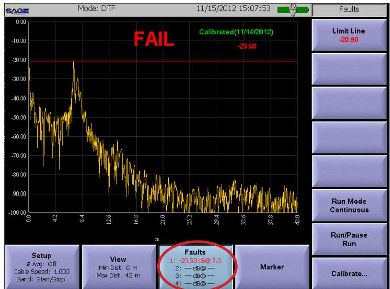
Figure 5.7.7 Distance to Fault Faults Menu
