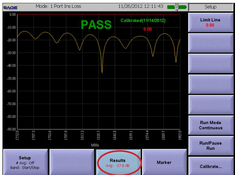
Figure 5.9.4 One Port Insertion Loss Results Menu
