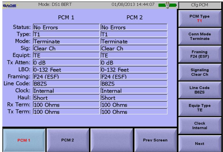
Figure 6.2.3 T1 PCM Configuration Menu
