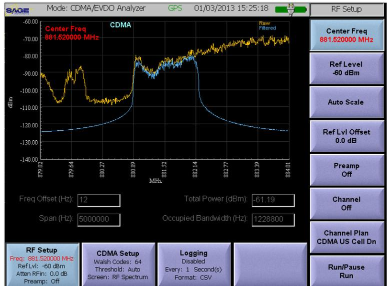
Figure 5.14.6 CDMA RF Spectrum Screen
