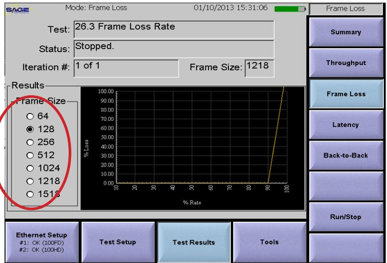
Figure 6.1.13 Frame Loss Test Results Screen
