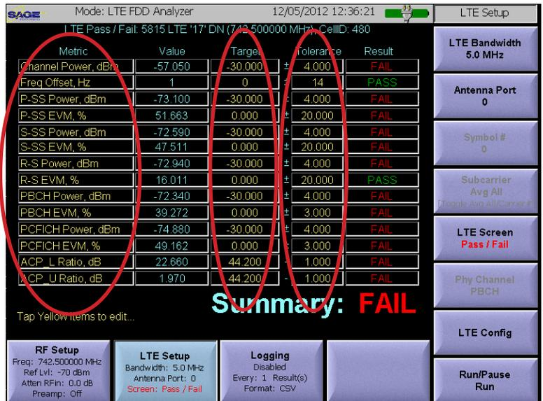
Figure 5.16.9 LTE Pass/Fail Screen
