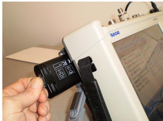
Figure 2.10 Removing/Inserting Battery
