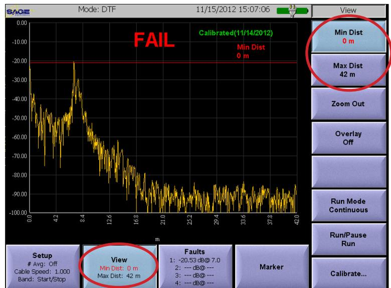
Figure 5.7.6 Distance to Fault View Menu
